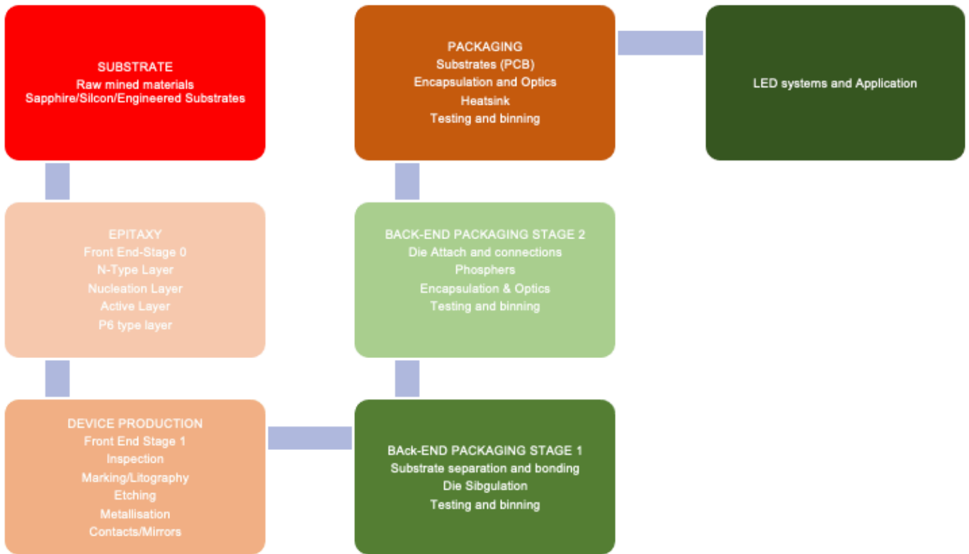
FIG 10. LED MANUFACTURING PROCESS-INFORMATION COURTESY OF ULSTER UNIVERSITY’S CREATIVE INDUSTRIES INSTITUTE
